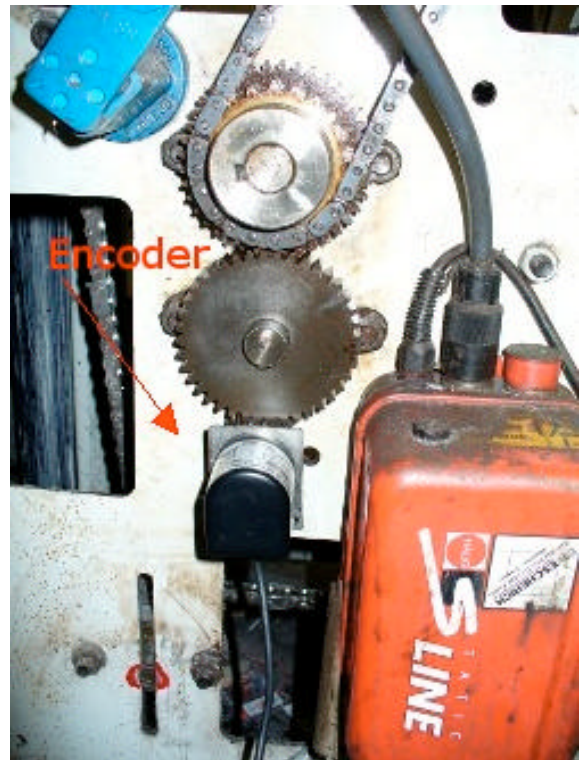
Example of encoder assembly on hot foil module transmission.
